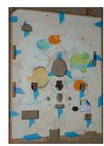
Reinstall your lost ball opening metal cover. Then you are ready to reinstall the ball track, be careful not to break the cotter pins.
