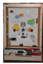
If you reuse the date stamp, get the plastic playing field cover and lightly sand the paper it down smooth on the back of the plastic behind the data stamp. Then apply double sided sticky tape to it, cut it out and place over the one on the playing field. Now reinstall all the playing field fetchers and start adjusting nails.
