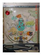
I first remove the glass and front playing tray, then the frame that held the glass is disassembled, I clean and polish all the parts, then reassemble them, the plastic part around the lock I clean and place in a Ziploc with the nails that held it in place then place in the front box.
